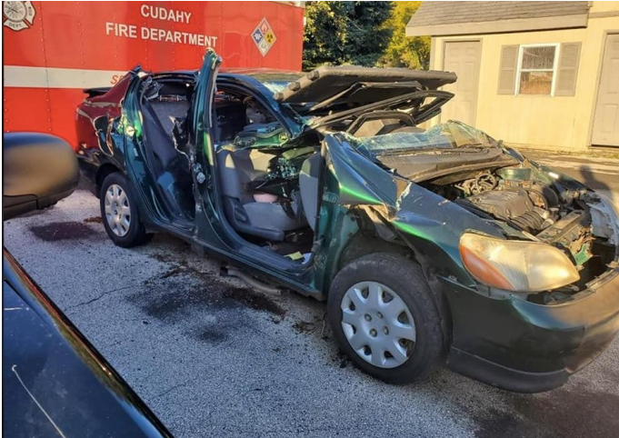
Training this week consisted of making vehicles open when they didn't want to and making them open where they normally don't. With the help of our extrication equipment (spreader, cutter, and rams) we are able to modify a vehicle to help with patient care and removal. Thankfully the CFD doesn't run into this type of rescue on a regular basis but it does happen. This training is extremely important because a fast extrication leads to better patient care. Thank you to Tim Wild and MT Towing for donating the vehicles!
